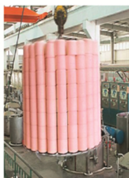
染色时加入抗菌剂 Dyeing with antimicrobial agents Ag+分布不均 contagious distribution Ag+外面多 More outside Ag+里面少 Little inside
